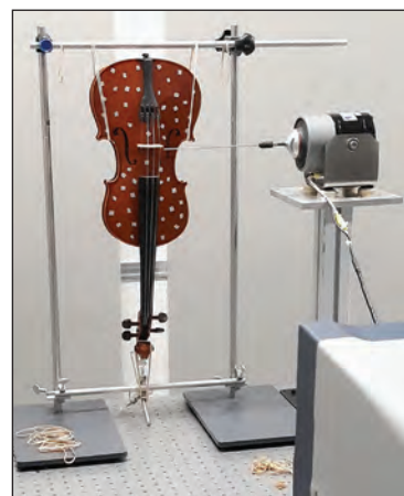
A violin is set up for acoustics testing, using a shaker and laser-scanning vibrometer.
